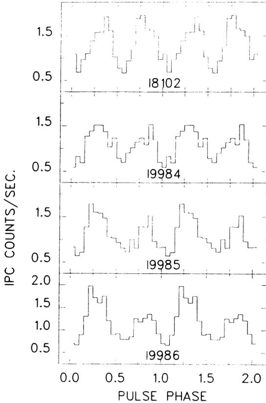
Figure 1: Pulsar light curves. Two cycles of the  $P = 6.978632$  sec. pulse are shown with 20 bins per cycle. Zero phase is set arbitrarily but all four data sets have been aligned in phase. Note that the modulated signal is sitting on top of a constant flux of approximately 0.5 counts/sec. The data shown is that in a box with a length of 4 arc min. per side centered on the pulsar. The background from the diffuse source is expected to contribute no more than 0.05 counts/sec in this field.
