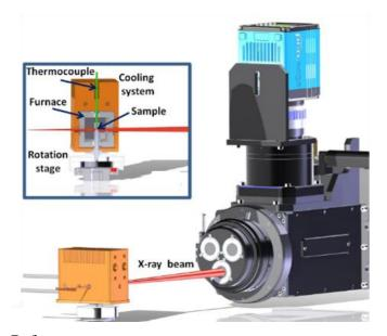
**Figure 1.** Schematic representation of the high temperature fast *in situ* nanotomography set up developed at ID16B ESRF beamline. The X-ray imaging microscope allows three scintillators to be used depending on acquisition conditions. The inset shows a cross section of the micro-heater exposing the cooling system, resistive furnace, quartz chamber and thermocouple.
