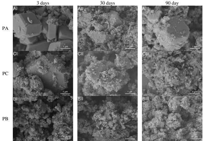
**Figure 1.** The microstructure of the lime putties PA, PB, and PC during their maturation and at the time 3, 30, and 90 days (HR-SEM JEOL JSM 6700F)
