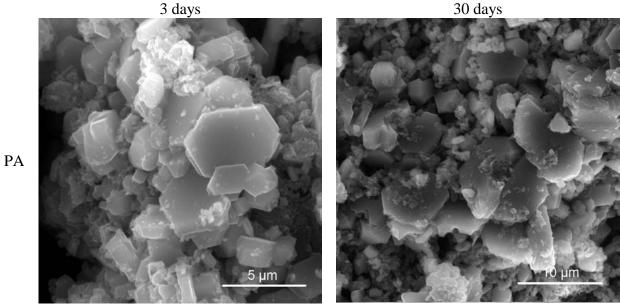
**Figure 2.** The microstructure of the lime putties PA during their maturation and at the time 3 and 30 days (ESEM AQUASEM II)
