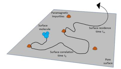
**Fig. 3.** Model of the two-dimensional translational diffusion of the proton species at the pore surface. The spin-bearing molecules (e.g. water) diffuse at the surface, sometimes reaching fixed surface paramagnetic impurities where the spins relax. The
