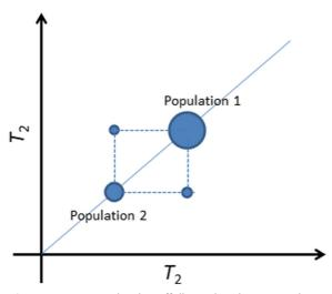
**Fig. 5.**  $T_2$ - $T_2$  maps showing off-diagonal peaks at an exchange time,  $t_E$ , indicating diffusive exchange between the two populations
