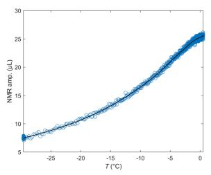
**Fig. 6.** Example of raw data recorded during NMRC experiments on the sample CW5 (Opalinus Clay). The line is a least square spline approximation used to calculate a smooth derivative dV/dT of the curve and produce the pore-size distribution according to Eq. 6
