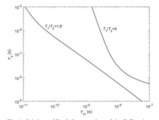
**Fig. 4.** Solutions of Eq. 2 for two values of the  $T_1/T_2$  ratio at 20.9 MHz;  $\tau_m$  is the correlation time of the dipole–dipole interactions at the surface governed by paramagnetic impurities and  $\tau_S$  is the surface residence time before desorption (see Fig. 3). A variation of the  $T_1/T_2$  ratio from 1.8 to 4 implies large variations of  $\tau_m$  and  $\tau_S$
