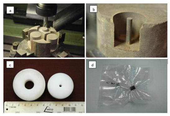
Fig. 9. Preparation of cylindrical cores for NMR studies. a Milling of cylindrical samples, b cylinder of 4 mm diameter for cryoporometry studies, c plastic rings into which the milled
