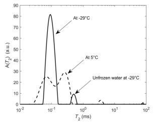
Fig. 8. Determination of the fluid volume in pores of <2 nm taking all components above 0.15 ms
