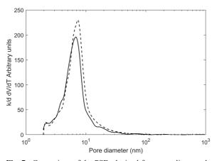
**Fig. 7.** Comparison of the PSD obtained from a zeolite sample with pure water (dashed line) and a potassium chloride solution of concentration 20 g/L (solid line)
