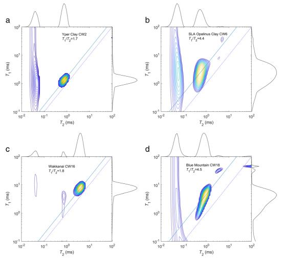
Fig. 13. Examples of  $T_1$ - $T_2$  maps for four formations with various  $T_1/T_2$  ratios. For the sample from the Blue Mountain Fm., the map was collected after KCl exchange. The dashed line indicates the diagonal  $T_1 = T_2$ ; the solid line indicates the  $T_1/T_2$  ratio of the mode
