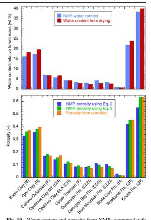
Fig. 10. Water content and porosity from NMR, compared with data from drying techniques and density measurements on adjacent materials
