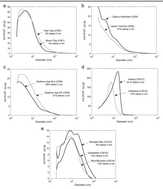
Fig. 11. Pore-size distributions from NMR cryoporometry. All samples contained the original porewater except for the Canadian samples (CW10, CW12, and CW18). When available, the amount
