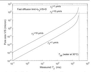
Fig. 1. Graphical representation of Eq. 1 with two extreme values of surface relaxivities. For completeness, the fast diffusion limit is also indicated
