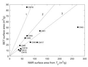
**Fig. 17.** Comparison of N<sub>2</sub> BET- and NMR-derived surfaces using the mode of the measured  $T_2$  distributions and a surface relaxivity of 1  $\mu$ m/s. The dashed lines indicates NMR values equal to or greater than by a factor of 1, 2, or 3
