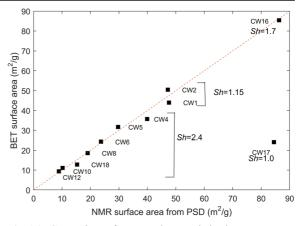
**Fig. 16.** Comparison of BET- and NMR-derived mesopore surfaces using the measured pore-size distributions and a shape factor of 2.4. To reconcile NMR and BET surfaces for CW1 and CW2, a shape factor of 1.15 would be required. The dashed line indicates the diagonal
