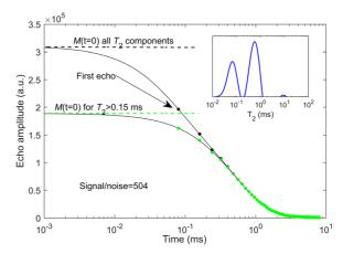
**Fig. 2.** Determination of the water content from NMR magnetization measurements (sample CW6, Opalinus Clay from Schlattingen). The solid line represents the inverse Laplace transform in the time domain and the circles represent the acquired data. The time axis is plotted using logarithmic scales to highlight the short time decay. The inset indicates the calculated  $T_2$  distribution using the recorded magnetization curve M(t)
