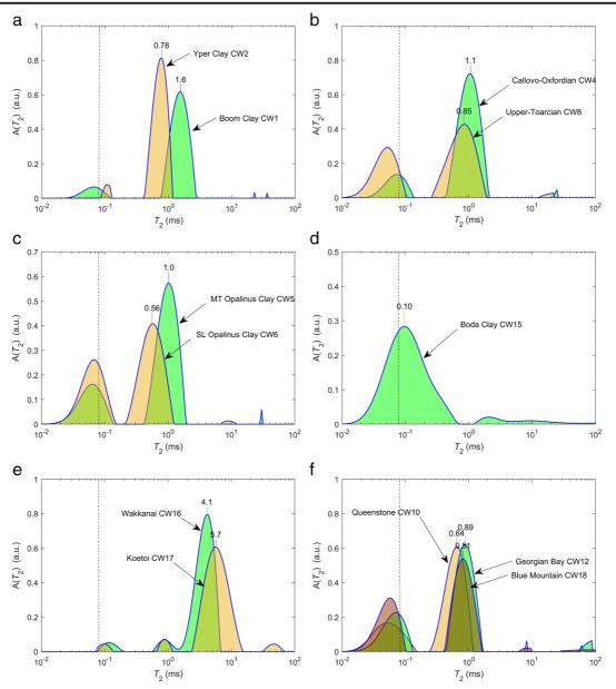
Fig. 12.  $T_2$  relaxation-time distribution for the 11 formations studied. The dashed line indicates the resolution limit. The value of the mode is indicated on top of each distribution. A( $T_2$ ) is the amplitude of the distribution at the value  $T_2$
