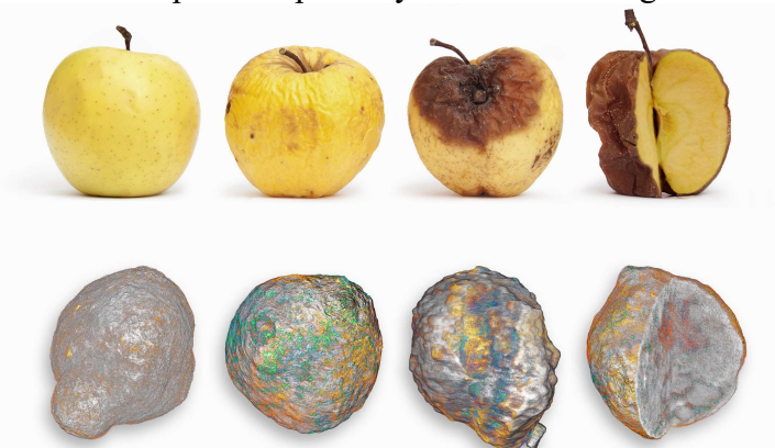
Figure 1. (top row) Pictorial to illustrate the life and death of a single Fluid Catalytic Cracking (FCC) particle by making the comparison with the rotting process of an apple; and (bottom row) 3-D TXM images of an FCC catalyst particle. From left to right, from a fresh catalyst particle to a catalyst particle rich in metal poisons, such as iron (orange-red) and nickel (green-blue). Reproduced from reference [10].
