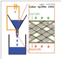
Schematic of the filtration device showing the three components used and the testing technique used for evaluation. NWs is nanowires and CNT is carbon nanotube. Reproduced with permission from *Nano Lett.* **10** (9) (2010) DOI: 10.1021/nl101944e; p. 3628.
