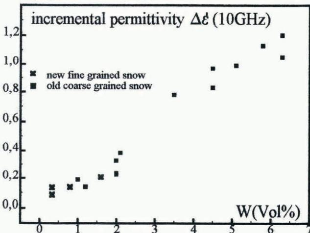
Fig. 10. Incremental permittivity  $\Delta\epsilon'$  for new fine-grained and old coarse-grained snow.
