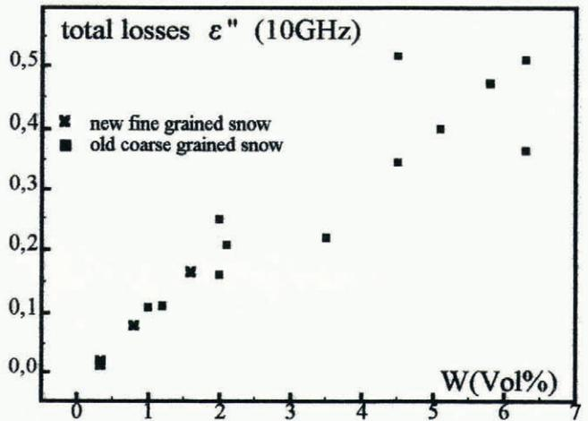
Fig. 11. Loss factor  $\epsilon''$  for new fine-grained and old coarse-grained snow.
