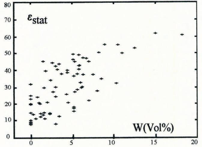
Fig. 7. Dependence of static dielectric constant on water content.
