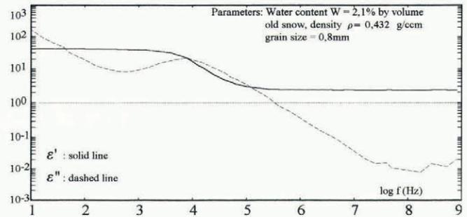
Fig. 3. Dielectric function of snow in the low and intermediate frequency regime.
