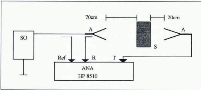
Fig. 2. Block diagram of the X-band measuring system. SO, sweeper oscillator; ANA, automatic network analyzer; S, sample; A, horn antennas; Ref, reference signal; R, reflected signal; T, transmitted signal.
