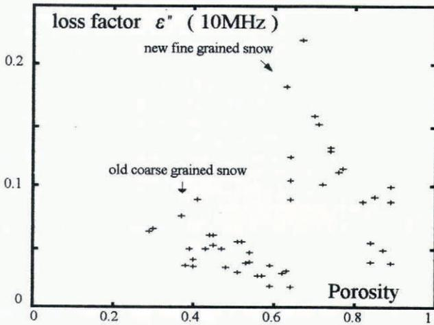
Fig. 9. Loss factor  $\epsilon''$  for new fine-grained and old coarse-grained snow.
