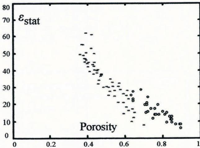
Fig. 6. Dependence of static dielectric constant on porosity. (Open symbols, new fine-grained snow; asterisks, old coarse-grained snow.)
