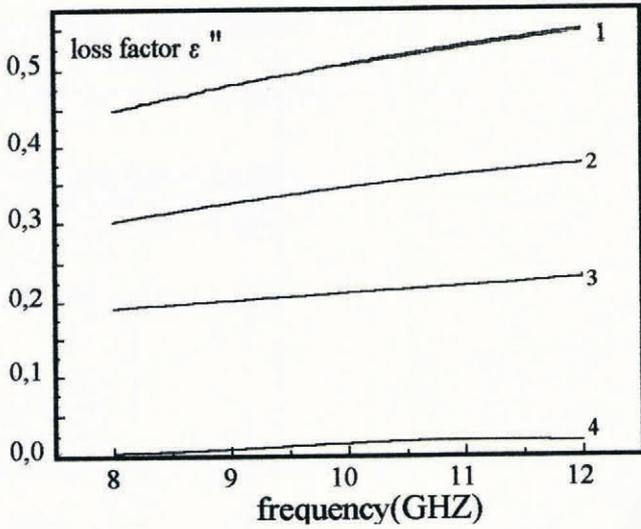
Fig. 5. Loss factor  $\epsilon''$  of snow between 8 and 12 GHz.
