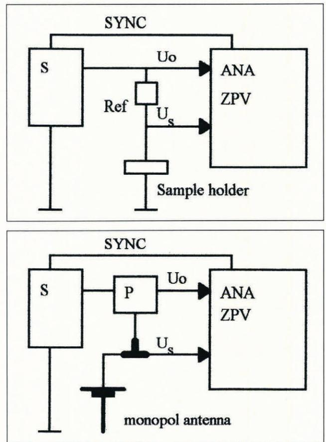
Fig. 1. Block diagram of the measuring systems. a, low-frequency. S, sweeper; ANA, automatic network analyzer ZPV; SYNC, synchronisation;  $U_o$ ,  $U_s$ , measured signals; Ref, reference impedance. b, intermediate frequency. S, sweeper; P, power splitter; ANA, automatic network analyzer ZPV;  $U_o$ ,  $U_s$ , measured signals.
