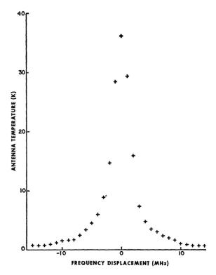
**Figure 1.2** The CO signal in the Orion Nebula as first detected. The plot shows the signal strongest at the exact frequency expected for CO in this source, falling dramatically within about ±10 MHz from that frequency. Credit: Wilson, Jefferts, and Penzias (1970); ©AAS, reproduced by permission.
