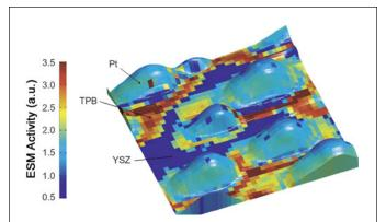
Map of electrochemical activity is overlaid onto the topography of Pt catalyst dots deposited on a YSZ surface. TPB indicates a triplephase boundary where the catalyst electrode is in contact with both the reactants and electrolyte. Reproduced with permission from Nature Chem. (DOI: 10.1038/NCHEM.1112; p. 707). © 2011 Macmillan Publishers Ltd.
