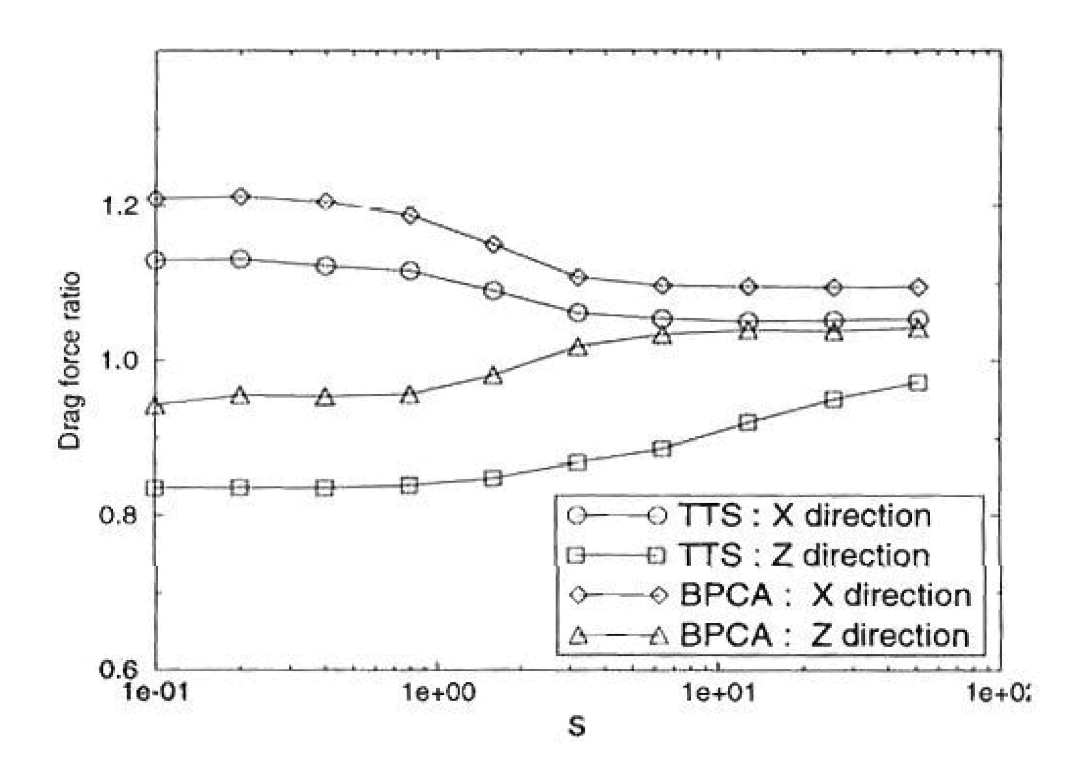
Figure 2. Same as Fig.1, but for the ratios of actual drag force on the target to that on an "area equivalent sphere".
