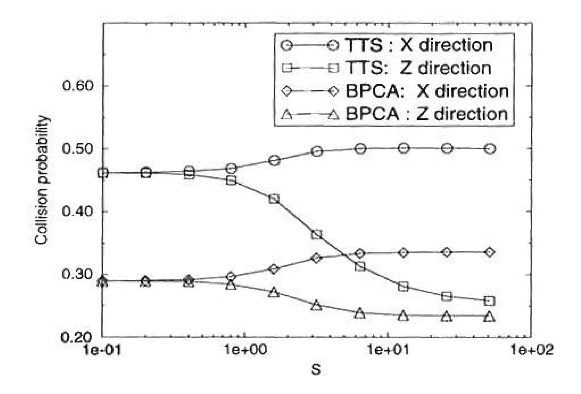
Figure 1. Fraction of incident molecules that experienced at least one collision. The horizontal axis represents S, the velocity of the aggregates normalized by the mean thermal velocity of the gas. The targets are two-touching spheres (TTS) and BPCA with 8 constituent particles.
