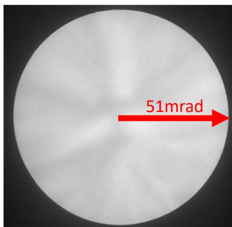
**Figure 2.** 40kV Ronchigram with 51mrad convergence semi-angle
