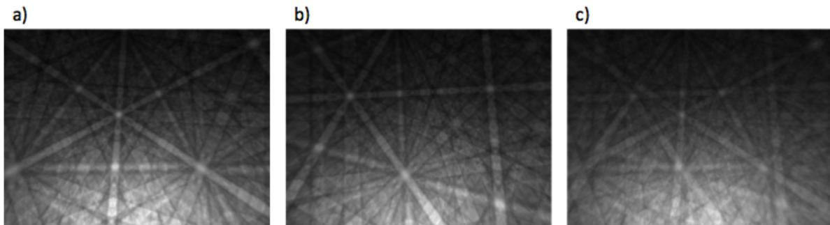
**Figure 2.** a) EBSD for Grain A, b) EBSD for Grain B, c) EBSD for the grain boundary between Grain A and Grain B where 50 percent of the electrons come from each grain.
