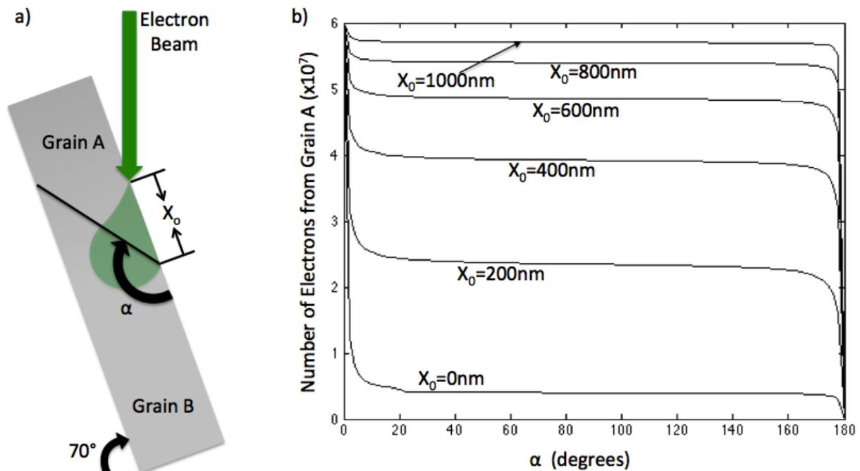
**Figure 1.** a) Sample geometry with a grain boundary inclination angle  $\alpha$  and distance  $X_0$  between electron beam incidence and boundary; b) number of electrons from Grain A vs. inclination angle  $\alpha$  for six different  $X_0$  values.
