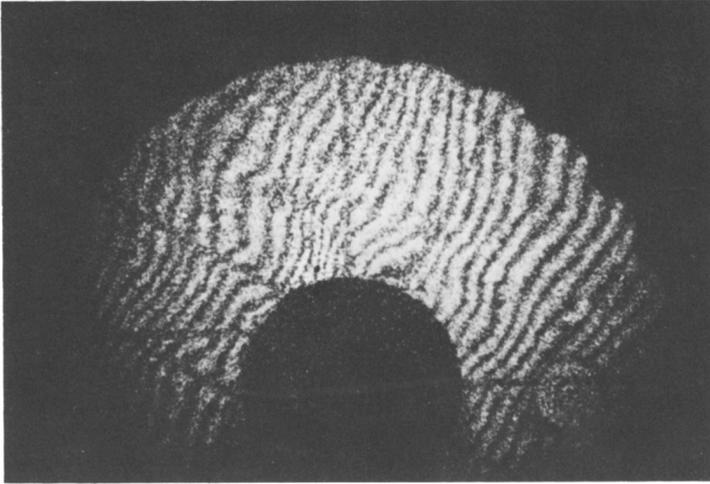
Figure 2 - Interferogram of Betelgeuse at  $\lambda = 5\,350 \text{ \AA}$  ( $\Delta\lambda = 90 \text{ \AA}$ ).
