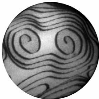
Figure 1. Stack of oval islands on a \text{TiO}_2 surface spawned from two screw dislocations.
