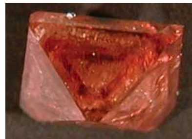
Figure 1. Single crystal of synthetic zircon, \text{ZrSiO}_4 , ~4 mm across, with 4–6 wt% ^{238}\text{Pu} (less than one week after synthesis).
