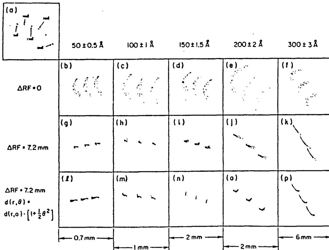
Figure 3. Oriental fan spectra. Here (a) is the gross wavelength map;  $\Delta RF$ =displacement between image plane and ruling focus; (b)-(f) have  $\Delta RF=0$ ; (g)-(k) have ruling focus optimized 7.2mm behind focal plane; (l)-(p) have also an optimized angular variation in groove spacing.
