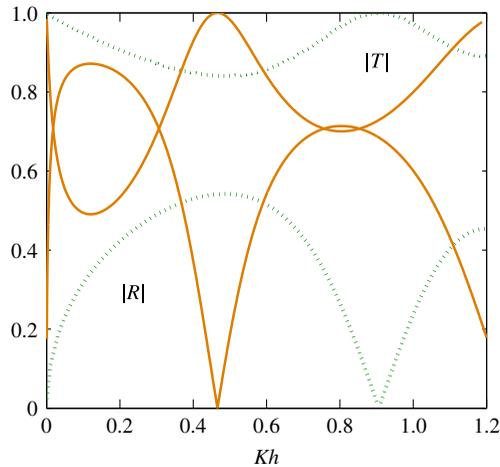
FIGURE 7. Plots of  $|R|$  and  $|T|$  against  $Kh$  with fixed values of  $\theta = 45^\circ$ ,  $b/h = 4$  and different values of  $c/h = 1$  ( $\cdots$ ) and 2 ( $-$ ).
