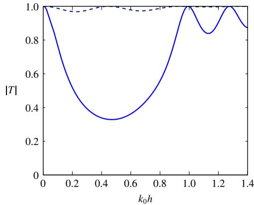
FIGURE 3. Plot of  $|T|$  against  $K_0 h$  with fixed values of  $c/h = 3$ ,  $b/h = 5$  and different values of  $\theta = 0^\circ$  (---) and  $45^\circ$  (—).
