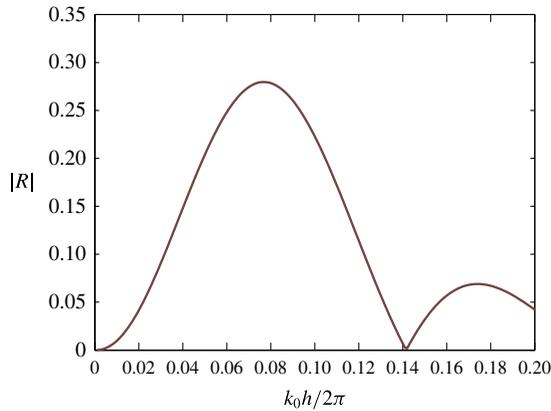
FIGURE 4. Plot of  $|R|$  against  $k_0 h / 2\pi$ ;  $c/h = 2$ ,  $b/h = 2.5$  and  $\theta = 0^\circ$ .
