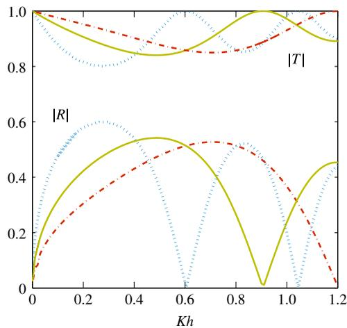
FIGURE 6. Plots of  $|R|$  and  $|T|$  against  $Kh$  with fixed values of  $\theta = 45^\circ, c/h = 2$  and different values of  $b/h = 2$  (---),  $3$  (—) and  $5$  (···).
