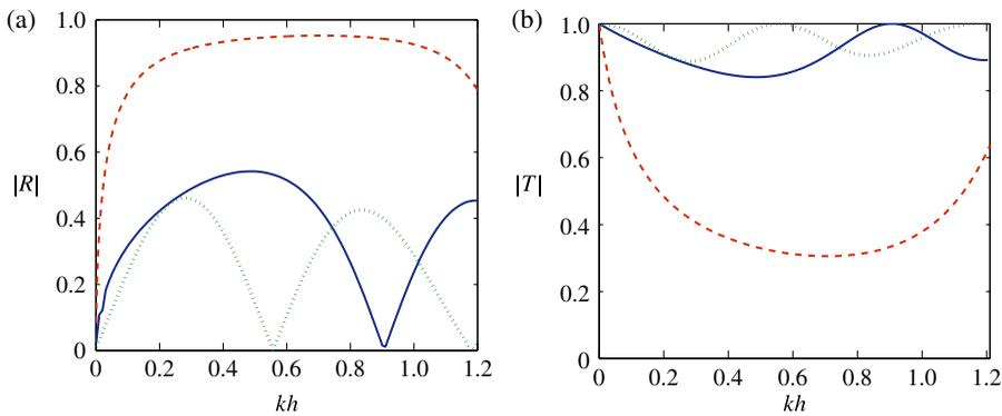
FIGURE 5. Plots of (a)  $|R|$  and (b)  $|T|$  against  $Kh$  with fixed values of  $b/h = 3, c/h = 2$  and different values of  $\theta = 30^\circ$  (---),  $45^\circ$  (···) and  $60^\circ$  (—).
