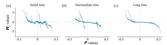
Figure 8. Non-vanishing momentum simulation. Values of P vs values of  $W_s$ . The end of each branch corresponds to a blob in figure 5. For example, at the initial time, a careful study reveals that the steep, overlapping branches just to the right of the y-axis match the two positive-negative blob pairs seen in the corresponding plot in figure 5.
