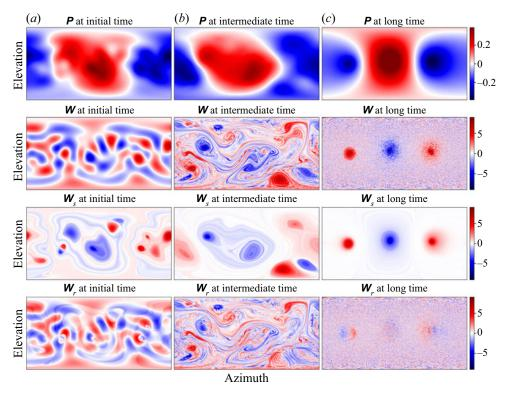
Figure 5. Non-vanishing momentum simulation. Progression of the stream matrix P and the components  $W_s$  and  $W_r$  of the vorticity matrix W. Initially,  $W_s$  and  $W_r$  are similar in nature, but they evolve so that  $W_s$  contains the large-scale condensates whereas  $W_r$  contains the small-scale fluctuations.
