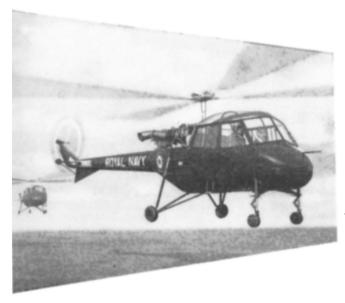
The P 531 has been designed to meet the demand for a compact turbine powered general purpose helicopter Good performance and carrying capacity versatility and ease of servicing are features of this functional aircraft
