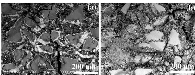
FIG 4: (a) and (b) BSE micrographs show the appearance of layer 3 in samples stored at room temperature and atmospheric pressure for three and five months, respectively.
