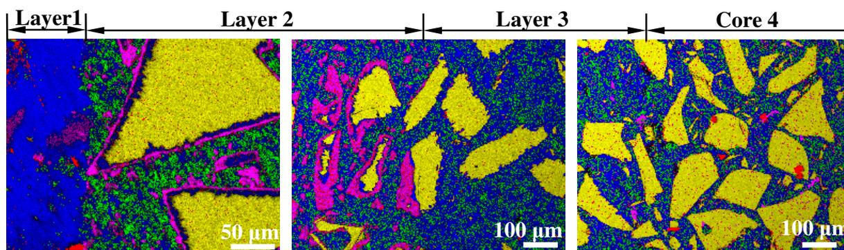
FIG 2: XEDS maps from cross-sectioned sample, layers 1 to 4. Color code: Al-blue, C-red, O-green, Si-yellow, Ti-magenta.
