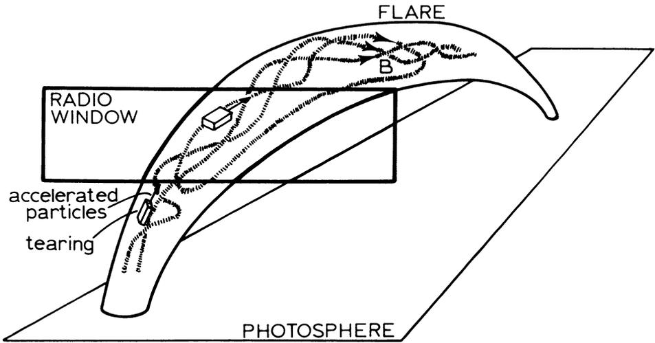
Figure 5. - Sketch of a flaring flux tube in which a few magnetic field lines have been drawn. Presumably tearing occurs in many thin regions two of which are indicated. Radiation from the tube at the plasma frequency can be observed with the radiospectrograph only within the "radio window".
