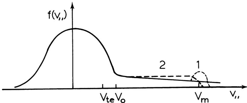
Figure 6. - The figure shows the "reduced" velocity distribution function (after integration over the velocity components perpendicular to the electric field direction).
