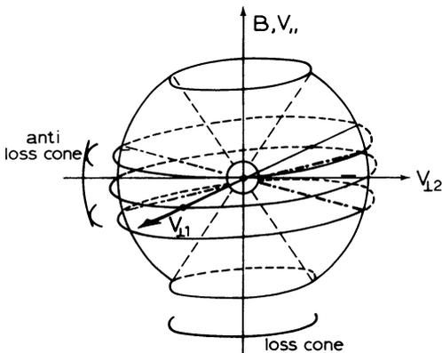
Figure 2. - The drawing shows the electron distribution function in velocity space. The small inner sphere represents the Maxwellian background distribution; from the outer sphere a loss-cone and an anti-loss-cone have been cut away.
