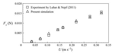
Figure 2. Comparison of the horizontal hydrodynamic drag  $F_x$  on the stem as a function of the inflow water current speed U in the first validation case of § 2.4:  $\square$ , the result from the experiment by Luhar & Nepf (2011);  $\triangle$ , the result from the present simulation.
