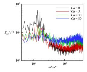
Figure 21. Averaged one-point temporal spectra over the canopy height for Ca = 0, 5, 30 and 80.
