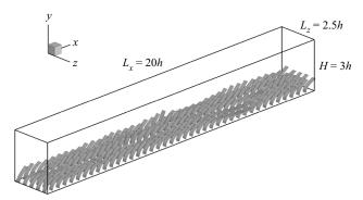
Figure 1. Configuration of the simulation set-up. The flow is driven by a pressure gradient along the streamwise direction over an evenly spaced  $40 \times 5$  array of stems. Here h stands for the height of an undeformed stem.
