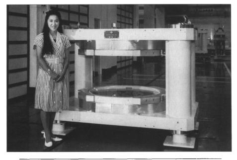
Figure 3. Permanent-magnet magnetic-resonance-imaging system produced by Sumitomo. Large disks of neo magnets at the top and bottom produce a vertical magnetic field in the gap of 0.2 T. The steel support structure withstands magnetic forces and provides a return path for the flux.
