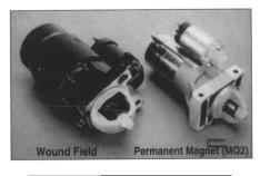
Figure 2. Showing the reduction in size of General Motors starting motors resulting from the use of neo magnets. (Magnaquench 2 is a dense unaligned magnet produced by pressing of rapidly solidified alloy.)
