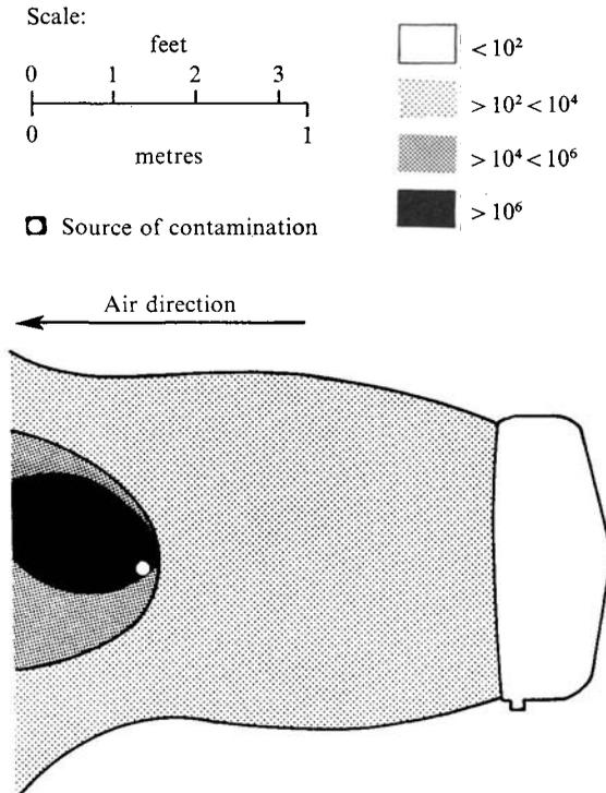
Fig. 2. Diagram showing the small amount of backflow and stagnancy from a source 1.4 m. from a large lamp.
