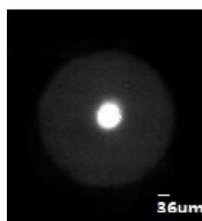
**Figure 3.** (a) The far-field pattern of the monicapillary; (b) The focused spot
