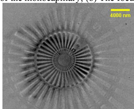
**Figure 4.** The TXM imaging of 100nm resolution target
