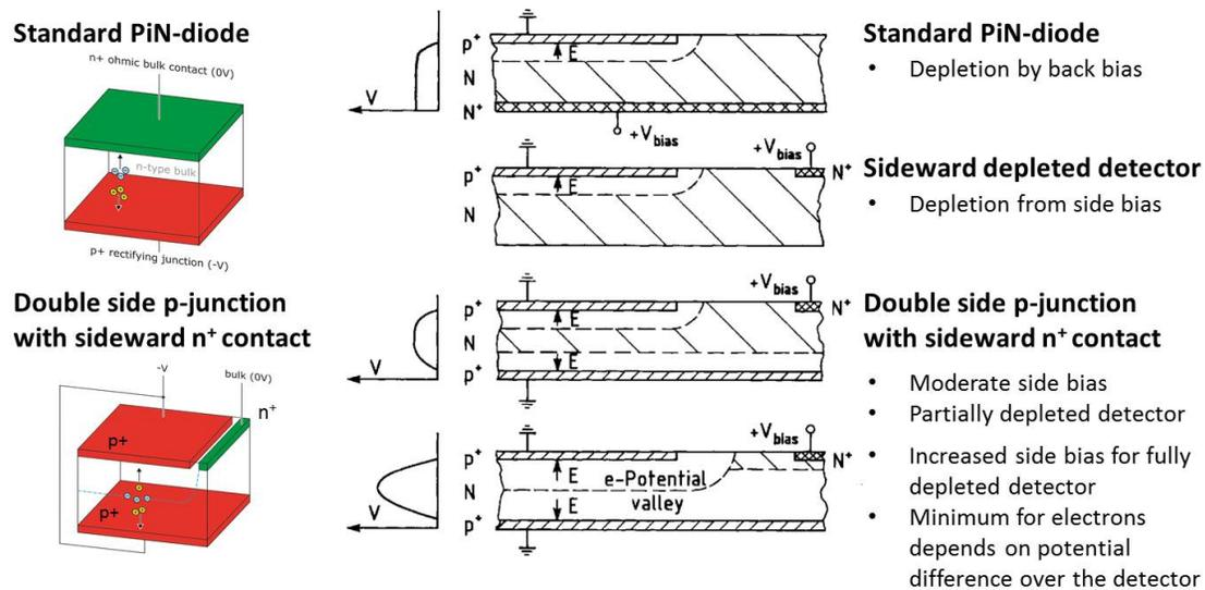
**Figure 1:** Principle of sideward depletion. The semiconductor wafer is fully depleted through a small n<sup>+</sup> contact reverse biased with respect to the p<sup>+</sup> implants realized on the two sides of the detector. The path of the charge carriers (left) and the electric potential (right) for different depletion geometries are shown. On the images on the right side, the hatched areas indicate the non-depleted sections. [4]
