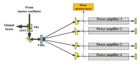
Figure 3. MOPA beam combination laser with the amplitude combining method using a VBG.
