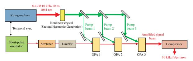
Figure 17. Schematic diagram of the generation of a fs/ps laser using the Kumgang laser as a pump source: OPA1–OPA3, optical parametric amplifiers.
