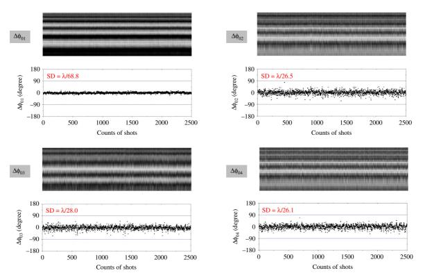
Figure 12. Measured phase fluctuation of the four-beam combination amplifier using an SBS-PCM with the wavefront dividing method.
