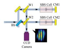
Figure 5. Experimental setup of the self-phase-locked SBS-PCM: BS, beam splitter; W1 and W2, wedges; CM1 and CM2, concave mirrors.
