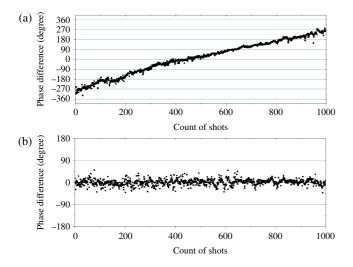
**Figure 8.** Experimental result of beam combination using an SBS-PCM and a feedback loop: (a) without operating the feedback loop and (b) with operation of the feedback loop.
