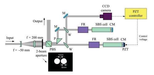
Figure 7. Experimental setup of beam combination using an SBS-PCM and a feedback loop: M, mirror; W, wedged window; CM, concave mirror.
