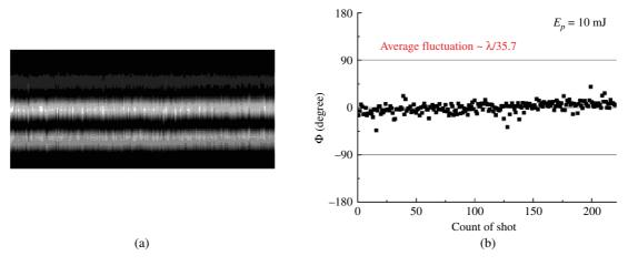
Figure 6. Experimental result of the self-phase-locked SBS-PCM. (a) A mosaic intensity pattern. It is generated by lining up one line of the intensity profile pattern recorded at each CCD image. (b) The measured relative phase. The standard deviation of the measured phase fluctuation is  $\lambda/35.7$ .
