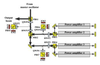
Figure 2. The MOPA beam combination laser with the amplitude combining method using PBSs: EM1–EM6, energy meters.
