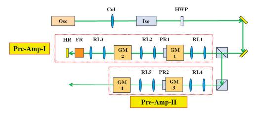
Figure 14. Schematic diagram of the pre-amplifier: RL1-RL5, relay lens pairs; PR1 and PR2, polarization rotators; HR, high-reflectivity mirror.
