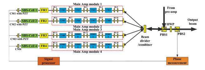
Figure 15. Schematic diagram of the main amplifier: RL1–RL20, relay lens pairs; CM1–CM4, concave mirrors.
