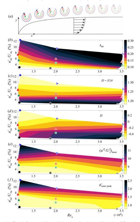
FIGURE 11. Trends for an evolving turbulent boundary layer subjected to different levels of freestream turbulence. Case REF  $\bullet$ ; A  $\blacksquare$ , green; B  $\blacktriangle$ , red; C  $\blacktriangleright$ , blue with fading colours indicating increasing streamwise distance from the grid.
