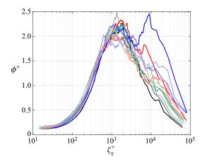
FIGURE 9. Normalized pre-multiplied velocity spectra at the near-wall spectral peak for cases REF solid black line, A solid green line, B solid red line, C solid blue with fading colours indicating increasing streamwise distance from the grid.
