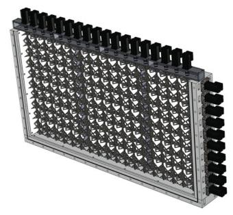
FIGURE 13. Three-dimensional view of the active grid at the water channel facility at the Norwegian University of Science and Technology.
