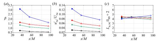
FIGURE 15. Analysis of the empirical parameter  $\beta$  introduced by Hancock & Bradshaw (1983) for cases REF •; A  $\blacksquare$ , green; B  $\blacktriangle$ , red; C  $\blacktriangleright$ , blue. Note that the scaling on these figures was chosen to represent equal changes in  $\beta$  and the two contributing parameters included in it.
