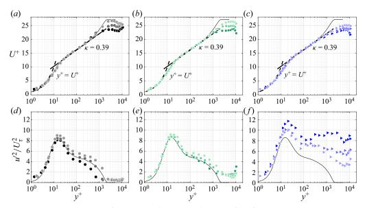
FIGURE 5. Development of mean velocity and variance profiles for cases REF •; A  $\blacksquare$ , green and C  $\blacktriangleright$ , blue with fading colours indicating increasing streamwise distance from the grid. DNS data of a fully developed canonical TBL at  $Re_{\tau} \approx 1990$  by Sillero *et al.* (2013) plotted as a reference solid black line.
