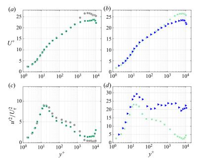
FIGURE 7. Comparison of TBL profiles with similar  $Re_{\tau}$ : (a,c) case REF at  $x/M = 95 \bullet$ , grey and case A at  $x/M = 35 \bullet$ , green; (b,d) case A at  $x/M = 95 \bullet$ , light green and case C at  $x/M = 35 \bullet$ , blue.
