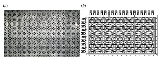
FIGURE 2. Biplanar active grid featuring square wings with holes. Viewed from the test section at full blockage and full schematic of the active grid.
