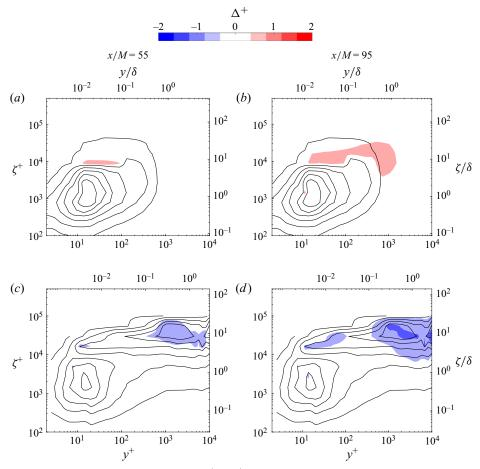
FIGURE 10. Net change  $\Delta^+ = (\phi^+ - \phi_0^+)/\phi_{0,max}^+$  in spectrograms at x/M = 55 and x/M = 95 for cases REF (a,b) and C (c,d) with respect to initial spectrogram at x/M = 35. The contour lines of the initial spectrogram are imprinted as a reference.
