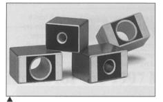
**EMI Filter Material:** Parite<sup>™</sup> from Paracon<sup>®</sup> provides up to 1,000 times more filtering than ferrite. The homogeneous crystalline material for cable and connector applications simultaneously forms both the magnetic core of a single turn inductor and the dielectric for coaxial capacitors. A line of D-subminiature backshells and custom overmold preforms using the filter system is available. **Circle No. 71 on Reader Service Card.**
