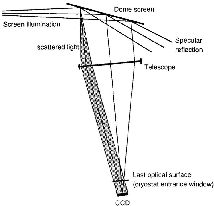
**Figure 1** Schema of dome flat fielding. Each element of the screen illuminates the whole CCD, and each point of the CCD is illuminated by all elements of the screen.
