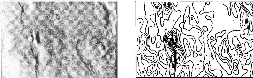
**Figure 3** Ratio of two MJUO *B* flat fields. One was obtained with the dome screen illuminated in the normal way, the other with only half the screen illuminated. The ratio image is presented in the same two ways as in Figure 2.
