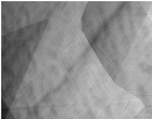
Figure 2. Optical micrograph of AlN crystal surface grown on-axis, as-received (0001) 6H-SiC substrate at 1780 °C and 400 torr for 40 hours with the magnification 100x (The real width of the crystal in above image is 1.0 mm).
