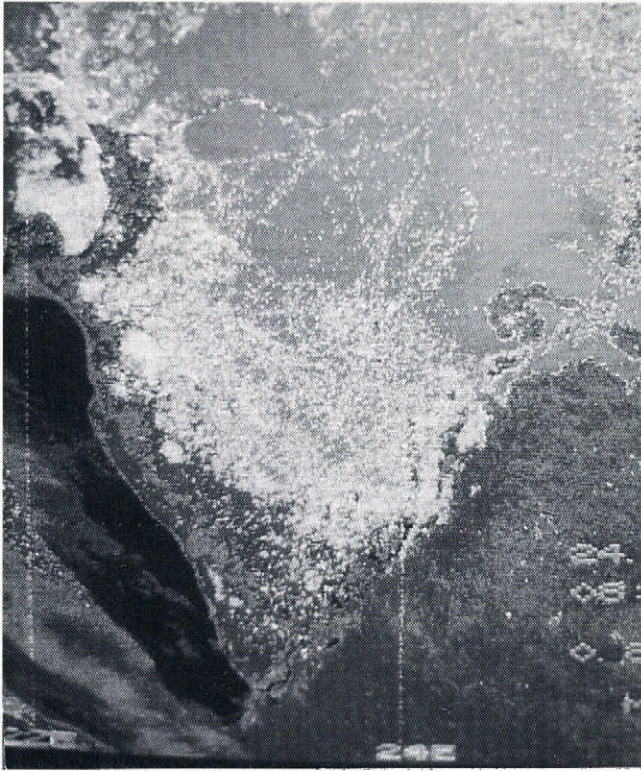
Fig. 3. Image over the Bay of Bothnia taken with Resource-01 MS-MC, 24 March 1990. Channel 4 (0.8–1.1 \mu\text{m} ).
