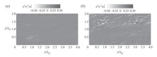
FIGURE 18. Instantaneous Reynolds shear stress on the horizontal plane,  $z^+ \approx 16$ , in the stratified flat case: (a)  $ft \approx 3$  during the initial transient, and (b)  $ft \approx 17$  at late time. The neutral value  $(u_{*N})$  of wall stress is used for normalization.
