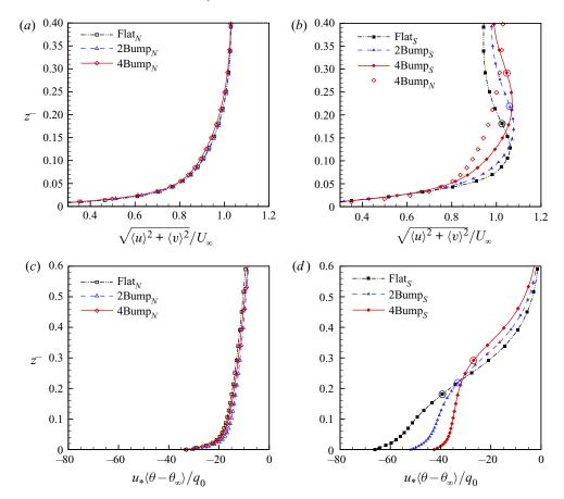
FIGURE 2. Mean velocity  $(\sqrt{\langle u \rangle^2 + \langle v \rangle^2}/U_{\infty})$  profiles: (a) neutral and (b) stratified cases. Potential temperature  $(u_{*_N}(\theta - \theta_{\infty})/q_0)$  profiles: (c) neutral cases where  $\theta$  is treated as a passive scalar, and (d) stratified cases. The large unfilled circle (right column) marks the time-evolving boundary-layer thickness  $(z = \delta_t)$ , defined by (3.7a,b).
