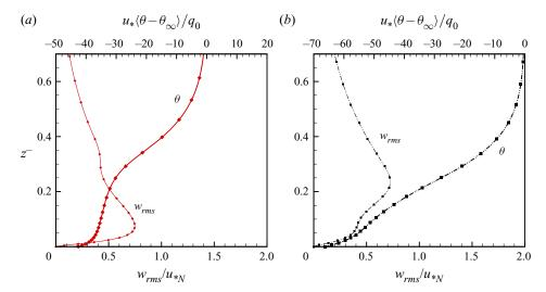
FIGURE 11. Comparison of rough and smooth-bottom cases in the context of Mahrt (1998) classification of the stable ABL. Potential temperature  $(\theta)$  and vertical r.m.s.  $(w_{rms})$  profiles: (a) 4Bump (-) case and (b) flat (- -) case. Normalization with  $u_{*N}$  and  $q_0$ .
