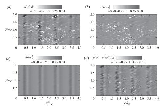
FIGURE 17. Instantaneous Reynolds shear stress and its components in the stratified 4Bump case at  $ft \approx 3$  on horizontal plane at the crest of the bump  $(z^+ \approx 16)$ : (a)  $u'w'/u_*^2$ , (b)  $u''w''/u_*^2$ , (c)  $\tilde{u}\tilde{w}/u_*^2$ , (d)  $(u'w'-u''w'')/u_*^2$ . The required time averages  $(\bar{u}$  and  $\bar{w}$ ) are computed using the evolution during 3 < ft < 6. The neutral value  $(u_{*N})$  of wall stress is used for normalization.
