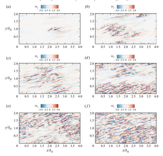
FIGURE 7. Vertical vorticity (normalized with  $u_{*N}/z$ ) contour at  $z^+ \approx 16$  in the stratified cases: (a,b) flat, (c,d) 2Bump and (e,f) 4Bump. Left column at  $ft \approx \pi$  and right column at  $ft \approx 4\pi$ .
