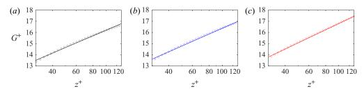
FIGURE 3. The mean velocity magnitude plotted in semi-logarithmic coordinates: (a) flat  $\kappa = 0.44$ , B = 5.82,  $z_0 = 0.0759$ , (b) 2Bump  $\kappa = 0.43$ , B = 5.77,  $z_0 = 0.0814$ , and (c) 4Bump  $\kappa = 0.40$ , B = 5.32,  $z_0 = 0.1187$ .
