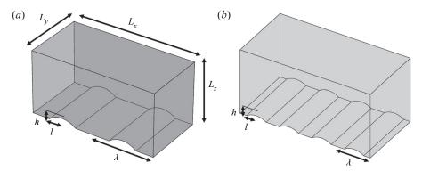
FIGURE 1. Schematic of the computational domain and surface roughness: (a) 2Bump and (b) 4Bump. Here  $L_x$ ,  $L_y$  and  $L_z$  are the domain size in the streamwise, spanwise and vertical directions, respectively. The wavelength of the harmonic function that generates the bump is  $\lambda = L_x/N_b$ , where  $N_b$  is the number of bumps. The half-length of the bump is  $l = \lambda/4$ .
