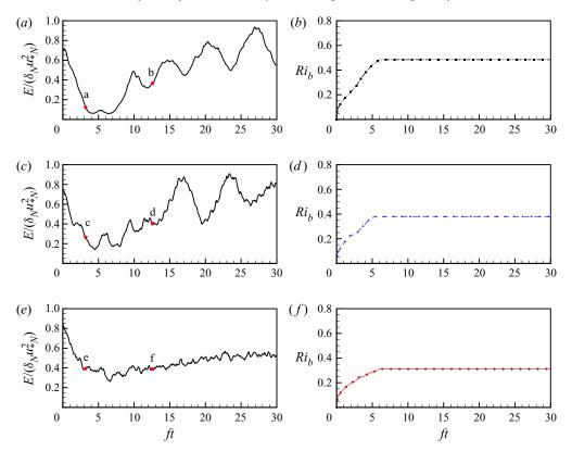
FIGURE 5. Overall behaviour of the stratified cases at  $Re_* \approx 700$ : (a,b) flat cases, (c,d) 2Bump cases and (e,f) 4Bump cases. The left column shows integrated TKE  $(E/(\delta_N u_{*_N}^2))$  and the right column shows the bulk Richardson number  $(Ri_b)$ . Points a–f (left column) mark the times of (a-f) in figure 7.
