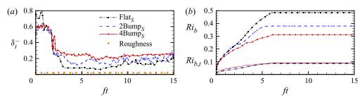
FIGURE 8. Time evolution of bulk quantities is contrasted among the different rough stratified cases: (a) local (in time) boundary-layer thickness and (b) bulk Richardson number  $(Ri_b)$  for flat -  $\blacksquare$  -, 2Bump -  $\blacktriangle$  -, and 4Bump  $\longrightarrow$  , and modified bulk Richardson number  $(Ri_{b,t})$  for flat, 2Bump - - - -, and 4Bump  $\longrightarrow$  . The roughness element height is also shown in (a).
