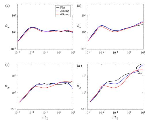
FIGURE 4. Normalized gradients ( $\Phi_m$  and  $\Phi_h$  defined by (3.2a,b)) of velocity (a,c) and temperature (b,d). Passive-scalar, unstratified cases are shown in the top row (a,b) and stratified cases in the bottom row (c,d).
