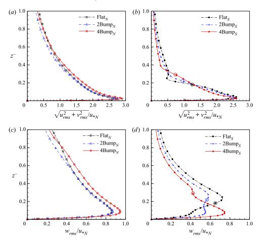
FIGURE 10. Profiles of velocity fluctuation statistics contrasted between neutral (a,c) and stratified (b,d) conditions: (a,b) horizontal velocity fluctuations  $(\sqrt{u_{rms}^2 + v_{rms}^2})$  and (c,d) vertical velocity fluctuations  $(w_{rms})$ . Open circle (right column) profile shows  $z = \delta_t$ .
