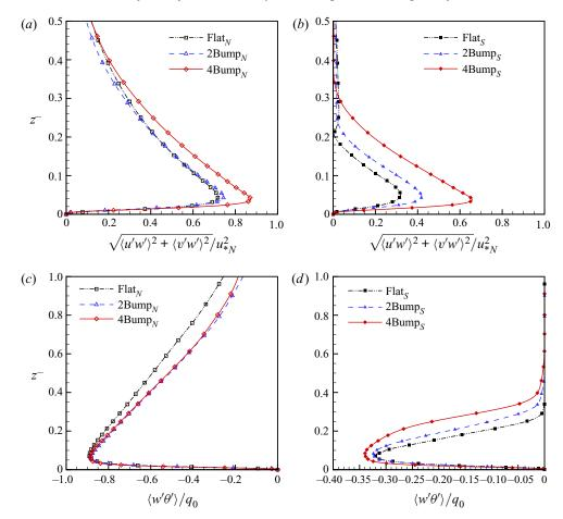
FIGURE 9. The effect of surface bumps on turbulent fluxes: (a,b) turbulent momentum flux  $(\sqrt{\langle u'w'\rangle^2 + \langle v'w'\rangle^2}/u_{*N}^2)$  profiles and (c,d) buoyancy flux  $(\langle w'\theta'\rangle)/q_0)$  profiles. Neutral situation shown in (a,c), and stratified counterpart in (b,d).
