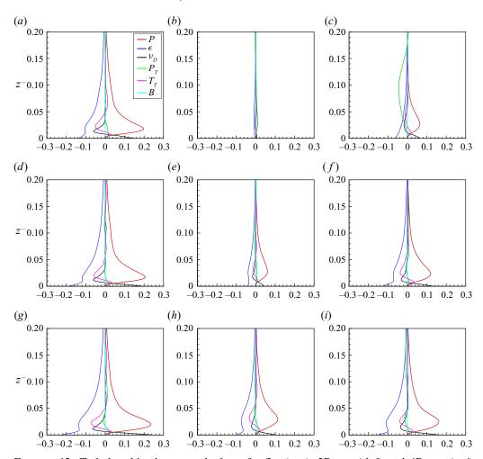
FIGURE 12. Turbulent kinetic energy budgets for flat (a-c), 2Bump (d-f) and 4Bump (g-i) cases at different times: ft=0 (a,d,g),  $ft\approx\pi$  (b,e,h) and  $ft\approx3\pi$  (c,f,i). Normalization with  $u_{*_N}^4/\nu$ .
