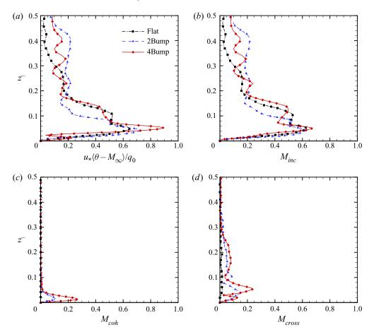
FIGURE 16. Decomposition of the turbulent momentum flux in the unstratified EBL: (a)  $M = \sqrt{\langle u'w' \rangle^2 + \langle v'w' \rangle^2}$ , (b)  $M_{inc} = \sqrt{\langle u''w'' \rangle^2 + \langle v''w'' \rangle^2}$ , (c)  $M_{coh} = \sqrt{\langle \tilde{u}\tilde{w} \rangle^2 + \langle \tilde{v}\tilde{w} \rangle^2}$  and (d)  $M_{cross} = \sqrt{\langle \tilde{u}w'' + u''\tilde{w} \rangle^2 + \langle \tilde{v}w'' + v''\tilde{w} \rangle^2}$ .
