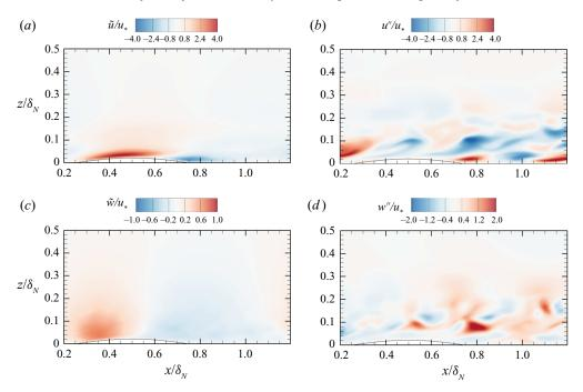
FIGURE 15. Vertical-plane snapshot of instantaneous velocity in the 4Bump unstratified case after the flow has reached a quasi-steady state: (a)  $\tilde{u}/u_*$ , (b)  $u''/u_*$ , (c)  $\tilde{w}/u_*$  and (d)  $w''/u_*$ . Flow is shown in the vicinity of a single bump.
