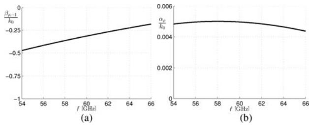
**Fig. 3.** (a) Normalized phase  $\beta_{\rho,-1}/k_0$  and (b) attenuation  $\alpha_\rho/k_0$  constants versus  $f$ , for the proposed LWA. The dispersion curves have been obtained through a method-of-moments (MoM) in-house code [28].
