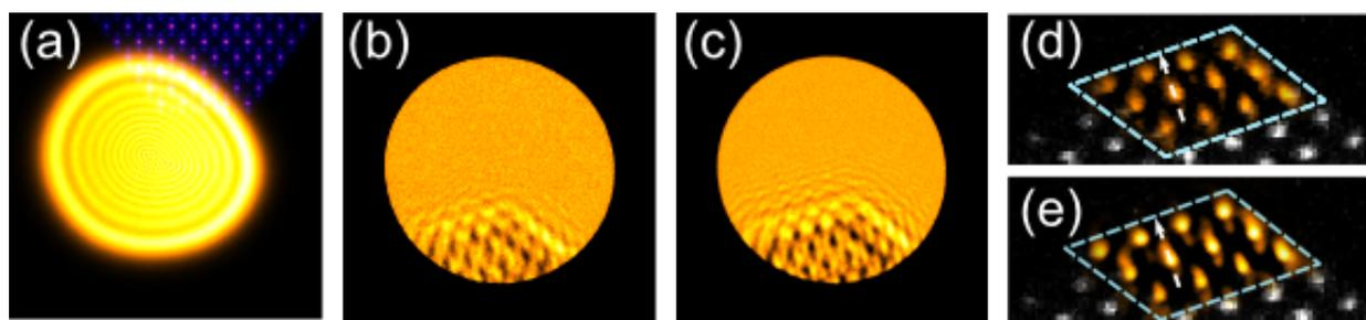
**Figure 2** (a) Probe sample configuration, and the corresponding (b) experimental and (c) simulated Ronchigrams. Reconstructed phase image of the specimen transmission function from (d) experiment and (e) simulation. The incident 300 keV electron probe was formed using an aperture of 24 mrad and a defocus of -80 nm.
