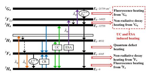
Figure 1. Energy diagram of a Tm:YAG crystal.
