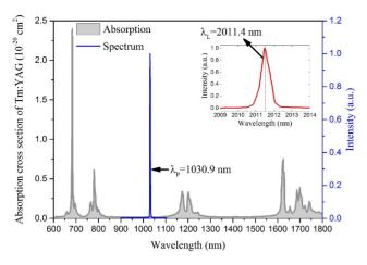
Figure 4. Absorption cross section of Tm:YAG and spectrum of pump light. Inset is the spectrum of output laser.
