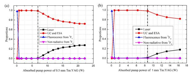
Figure 9. Proportions of all the transitions for (a) 0.5 mm Tm:YAG disk laser and (b) 1 mm Tm:YAG thick disk laser under the lasing condition.
