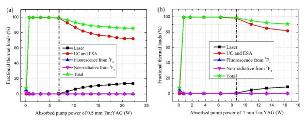
Figure 10. Fractional thermal loads of all transitions for (a) 0.5 mm Tm:YAG disk laser and (b) 1 mm Tm:YAG thick disk laser under the lasing condition.
