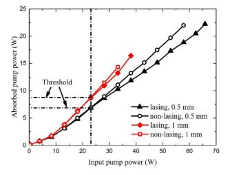
Figure 5. Absorbed pump power of a Tm:YAG crystal versus input pump power under non-lasing and lasing conditions for 0.5 and 1 mm thickness of gain medium.
