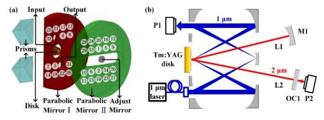
Figure 3. Layout of the (a) 20-pass pumping head and (b)  $2 \mu m$  Tm:YAG disk laser multi-pass pumped by a  $1 \mu m$  laser.
