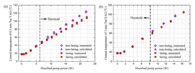
Figure 8. Central temperature of (a) 0.5 mm Tm:YAG disk and (b) 1 mm Tm:YAG thick disk versus absorbed pump power under lasing and non-lasing conditions.
