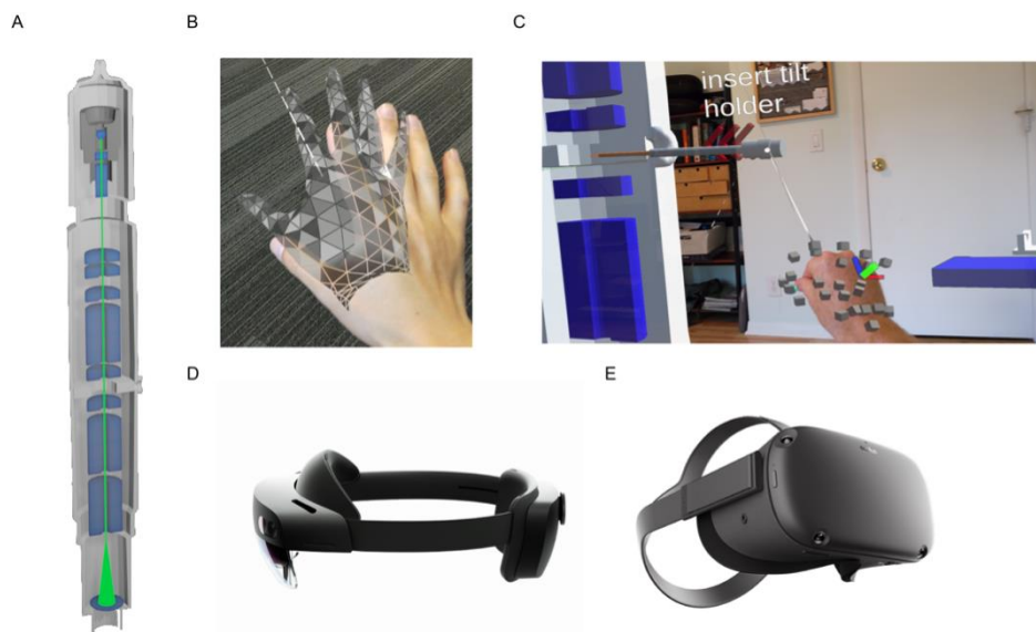
Figure 2. Figure 2: 3D models and content can be embedded in the web portal for virtual lab content. The 3D models such as the TEM column above can be created in open-source software such as Blender and exported as glTF format to be included in WebXR components (A). Articulated hand-tracking is a new input modality possible with the latest generation of devices (B). We are testing using the hand-tracking as an intuitive way to engage with training simulations such as loading a TEM column with a sample. Here shown through the
