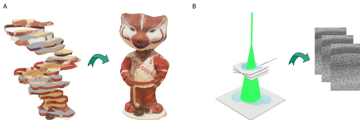
Figure 1. Figure 1: A tomographic reconstruction of UW-Madison's Bucky as a 3D volume from a series of image slices (A). In cryo-electron tomography, detailed models of frozen biological samples are reconstructed from projected images on a detector plate recorded at a series of tilt angles.
