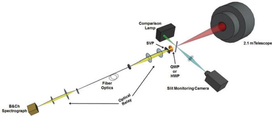
**Figure 1.** Optical layout of the polarimeter module for the B&Ch spectrograph at the 2.1-m telescope of the San Pedro Martir Observatory.
