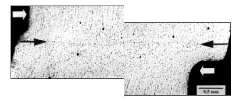
Figure 1. Cross section of an Al-6082 bond with sinusoidal interface (shown by black arrows) using the temperature gradient bonding method and which subsequently withstood 251 MPa in a shear test. White arrows show the direction of the applied shear force and the extent of lateral plastic deformation.
