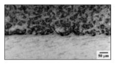
Figure 2: Cross section of a dissimilar joint of Al-6082 alloy and an Al/SiC particulate composite made using the temperature gradient bonding method.
