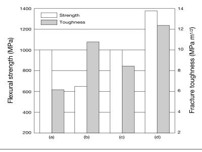
Figure 2. Comparison of the mechanical properties of (a) conventional silicon nitride, (b) conventional toughened silicon nitride, (c) seeded silicon nitride, and (d) seeded and tape cast silicon nitride.
