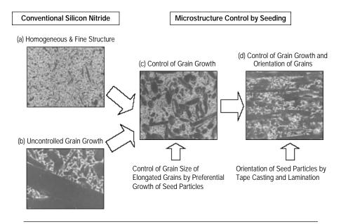
Figure 1. Microstructures of (a) conventional silicon nitride, (b) conventional toughened silicon nitride, (c) seeded silicon nitride, and (d) seeded and tape cast silicon nitride.
