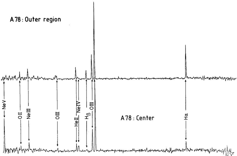
Fig. 1. The spectrum of A78. The above spectrum (a) shows a region 30" SW of the center in the outer nebula, while the lower spectrum (b) is a region near the center. Note the weakness of H $\beta$  near the center.
