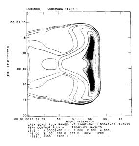
Fig. 3 Radio surface brightness distribution of a hotspot seen edge-on, as determined from hydrodynamic simulations. Synchrotron emissivity is assumed to be proportional to the gas pressure squared within the jet working surface (Fig. 2). The map is smoothed and displayed using AIPS shading and contouring algorithms.
