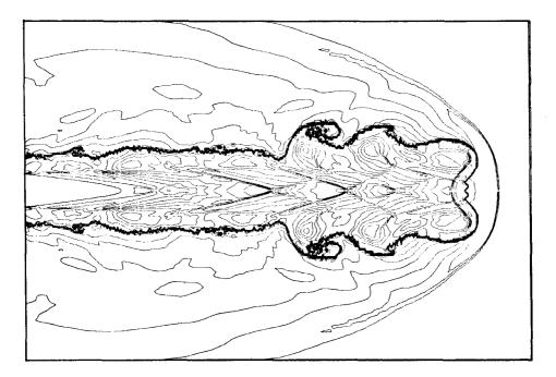
Fig. 2 Hydrodynamical simulation of an axisymmetric, pressure-matched, supersonic (M=6) jet of lower than ambient density ( $\eta$ =0.1), from [17]. A computational mesh of 640 axial by 75 radial zones is used; 20 zones span the beam radius at the inlet at left.
