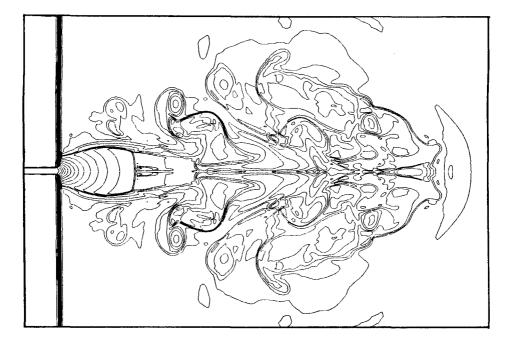
Fig. 4 Disruption of a supersonic (M=1.5) jet caused by a rapid decrease in ambient pressure. Overexpansion and reconfinement creates a Mach disk shockwave (highlighted) within the jet beyond which the flow is subsonic. This mechanism may be responsible for producing the plume-like tails in radio galaxies. A computation mesh of 500 axial zones by 150 radial zones is used; 5 zones span the initial beam radius.
