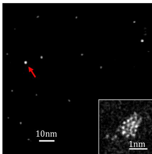
FIG. 1. Typical HAADF-STEM image of MP-Au<sub>38</sub> clusters. The cluster indicated with the arrow is an aggregate from the monomers. The inset displays a high-resolution atomic structure image of MP-Au<sub>38</sub> monomer.
