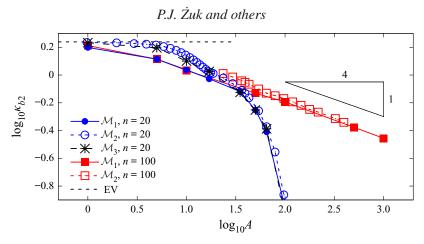
Figure 15. Comparison of three bead models of a flexible fibre. The maximum curvature  $\kappa_{b2}$  vs. bending stiffness *A*, evaluated with the use of the models  $\mathcal{M}_1$  (filled symbols),  $\mathcal{M}_2$  (empty symbols) and  $\mathcal{M}_3$  (stars). The EV limit is marked as the horizontal dashed line.
