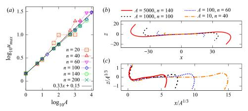
Figure 9. Maximum deflection  $u_{max}$  of the fibre tip, defined as  $z_1(t_{max})$  at the time  $t_{max}$  of the first maximum, evaluated numerically from the bead model  $\mathcal{M}_1$ . (a)  $u_{max}$  as a function of A for different n, with the approximate scaling  $\propto A^{1/3}$ . (b) Shapes of fibres at  $t_{max}$  for different A and n. (c) Rescaled shapes of fibres from (b), translated to overlay the bending left ends.
