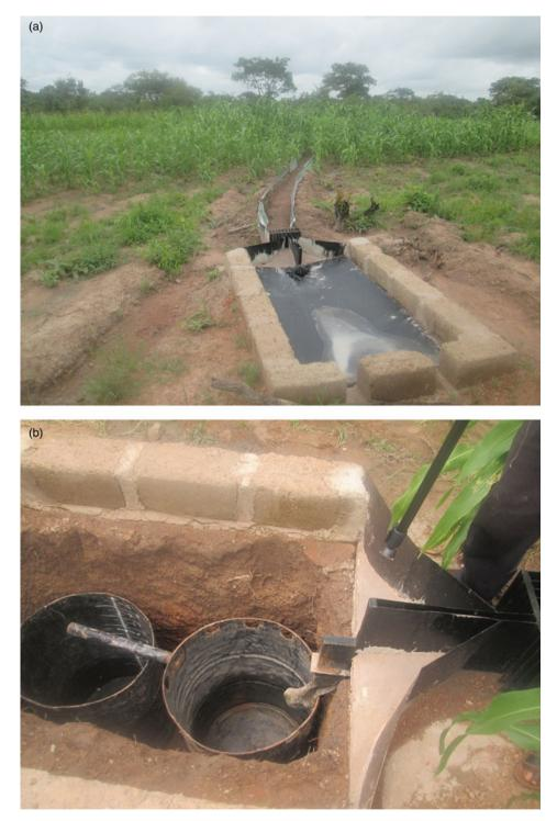
Fig. 3. (a) Structural layout of water runoff and erosion monitoring device and (b) water runoff collection chamber.
