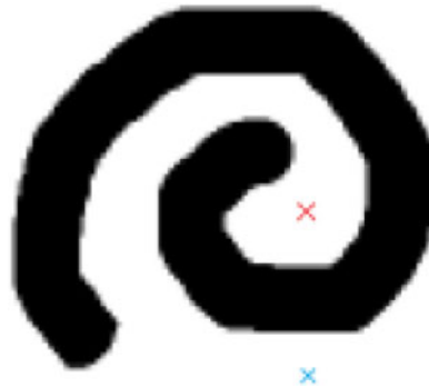
Fig. 4. The barrier contains both concave and convex sub-edges. If we consider the barrier as an edge rather than divide it into sub-edges, as shown Fig. 5, then we cannot reach the target inside the barrier using a tangent to the entire edge from outside.
