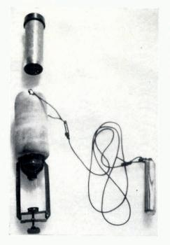
Fig. 1. Centrifuge for separating water from melting snow (see E. R. LaChapelle, p. 769)
