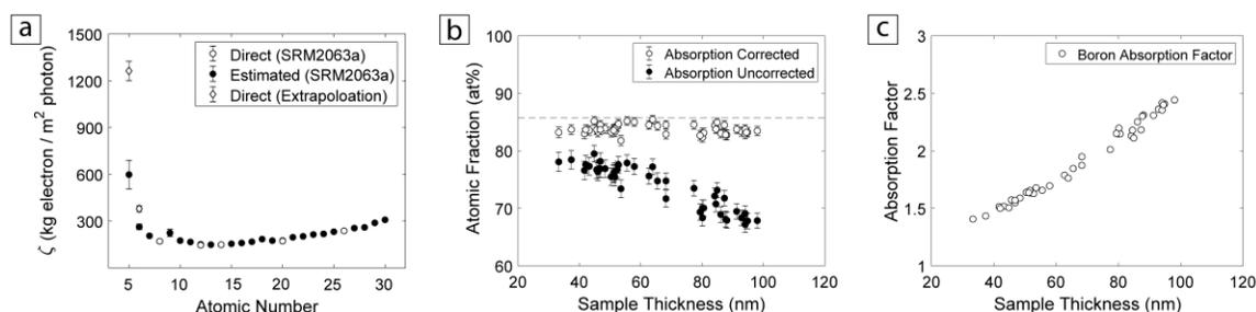
**Figure 1.** Summary of (a)  $\zeta$ -factors used throughout this study, (b) B concentration vs sample thickness measured from a  $\text{SiB}_6$  standard which was used as validation, and (c) a summary of the associated absorption correction factors applied to the B K-line X-rays where a 250% correction was applied at a sample thickness of 100 nm.
