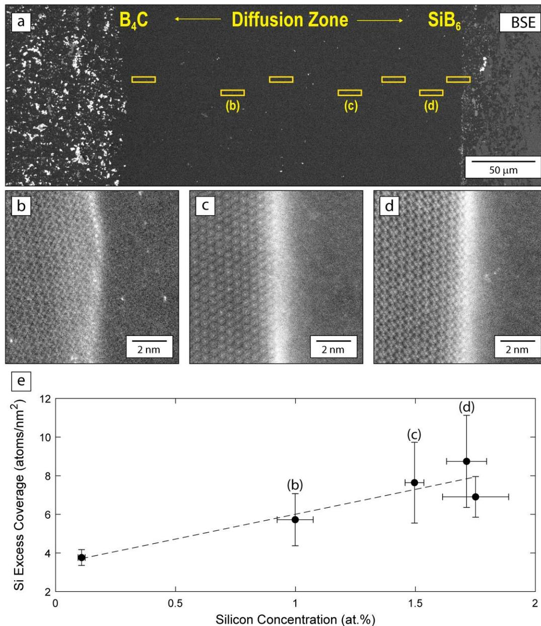
**Figure 2.** Summary of analytical results from the (a)  $B_4C:SiB_6$  diffusion couple where multiple thin specimens (shown in yellow) were extracted for  $\zeta$ -microanalysis, (b-d) high-angle annular dark field micrographs showing minimal differences in grain boundary structure from different regions of the diffusion zone, and (e) grain boundary segregation dependence of Si concentration in the bulk boron carbide lattice.
