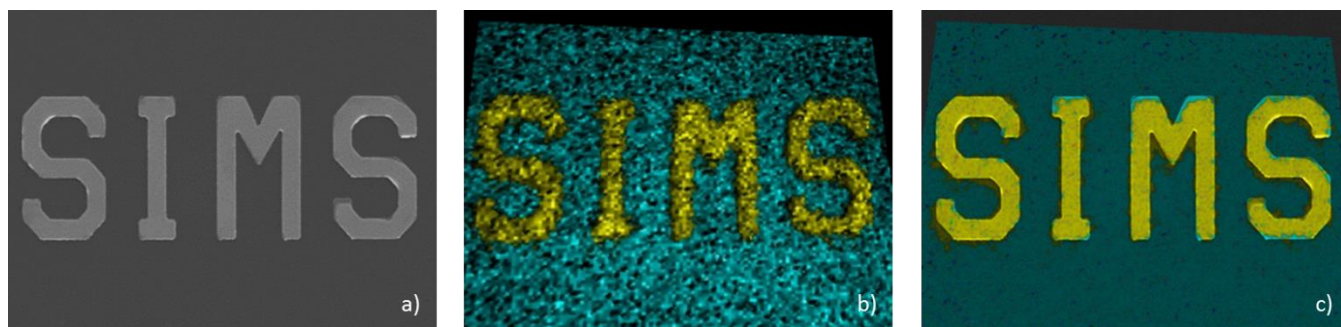
Figure 1. (a) SEM image of the word “SIMS” on an image standard; (b) SIMS image of the same feature where yellow represents the Si distribution and cyan represents the Ta distribution. The input images were registered using the MATLAB Image Processing Toolbox; (c) result of image fusion via pan-sharpening of (a) and (b).
