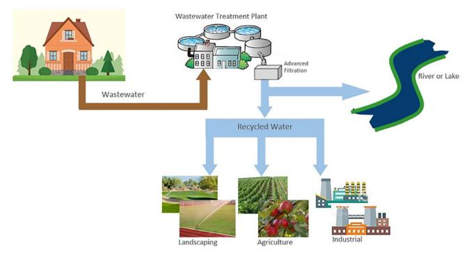
Fig. 1. Illustration showing the process whereby a wastewater treatment plant equipped with advanced filtration turns wastewater into municipal recycled water (figure presented in Section 3 of the survey).
