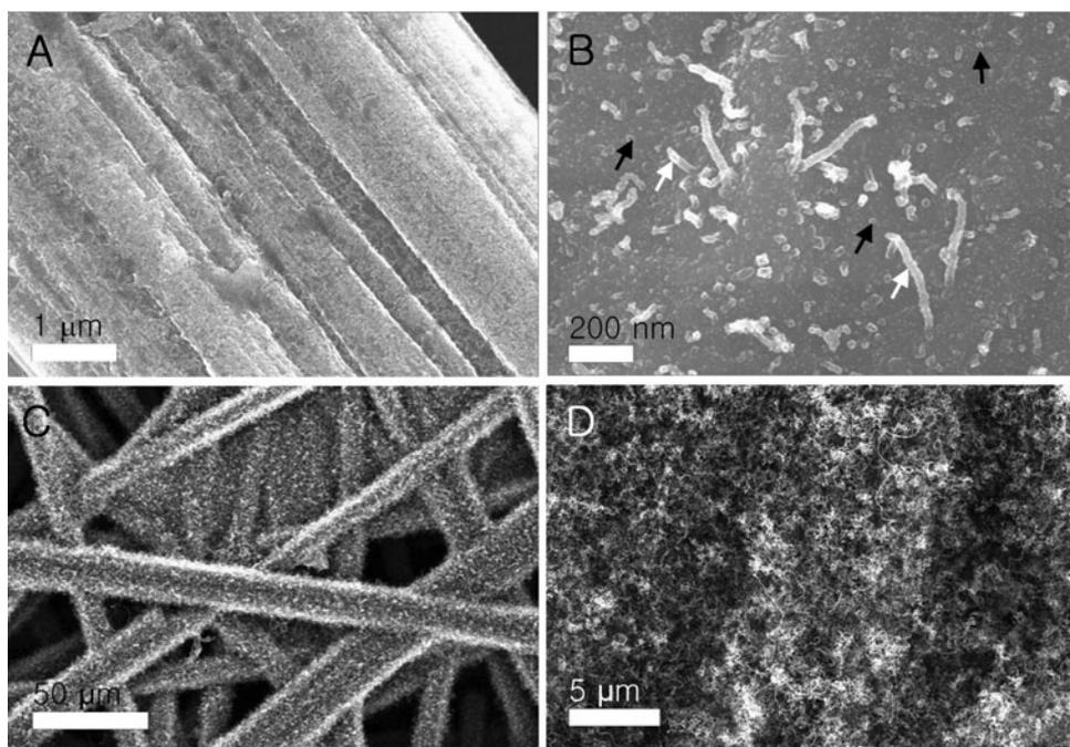
**Figure 1.** SEM images: (A) Ni thin film coated on carbon fiber paper (CFP), (B) tiny nanowires formed after exposure to ethanol for 30 s, and (C, D) mature carbon nanowires grown on the surface of the CFP.
