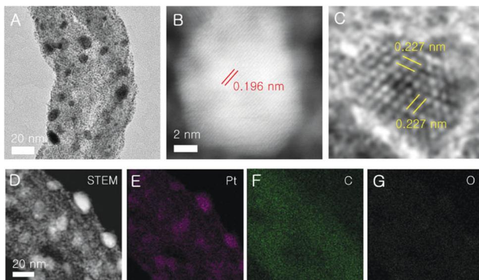
**Figure 4.** TEM, STEM, and EDX mapping images of the Pt-CNW hybrid materials: (A) Pt nanoparticles decorated on the CNWs, (B, C) lattice structures of Pt nanoparticles with diameter in the range of 2–10 nm, (D–G) EDX mapping images. TEM, transmission electron microscopy; STEM, scanning transmission electron microscopy; EDX, energy-dispersive X-ray spectrometry; CNW, carbon nanowires.
