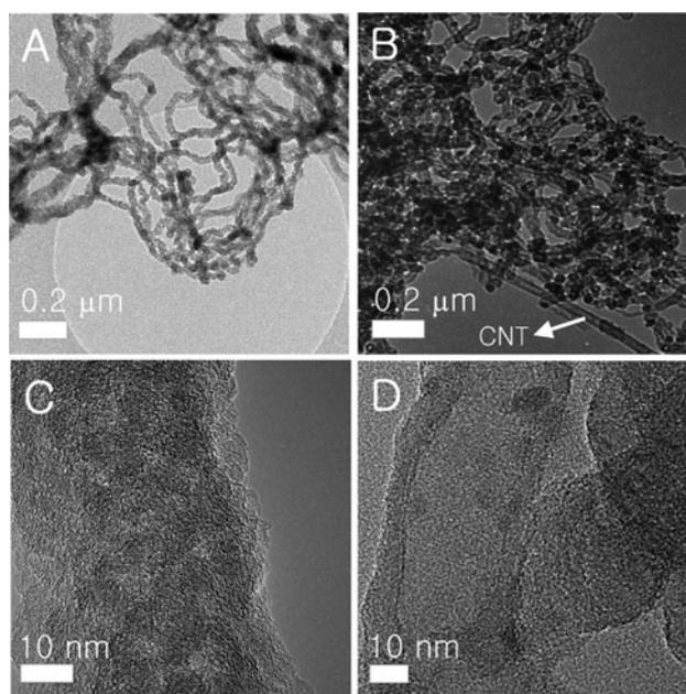
**Figure 3.** TEM and HRTEM images of CNWs grown at (A, C) 600°C and (B, D) 700°C. TEM, transmission electron microscopy; HR-TEM, high-resolution transmission electron microscopy; CNW, carbon nanowires.
