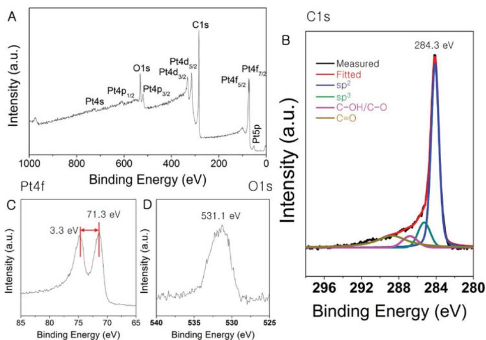
**Figure 5.** X-ray photoelectron spectroscopy spectra of the Pt-carbon nanowires hybrid materials: (A) survey and detailed scans of (B) C 1s, (C) Pt 4f, and (D) O 1s.
