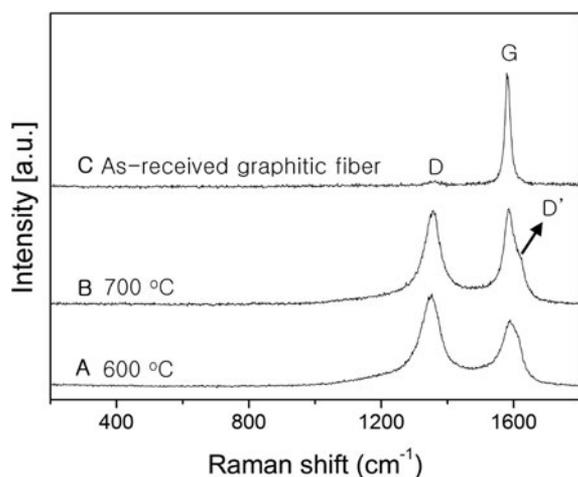
**Figure 2.** Raman spectra of carbon nanowires grown at different synthesis temperatures: (A) 600°C and (B) 700°C; (C) Raman spectrum of as-received carbon fiber paper.
