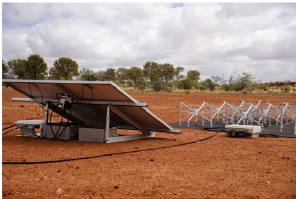
Figure 4. A Phase II long baseline tile. The batteries and BFIF systems are located under the solar panels.
